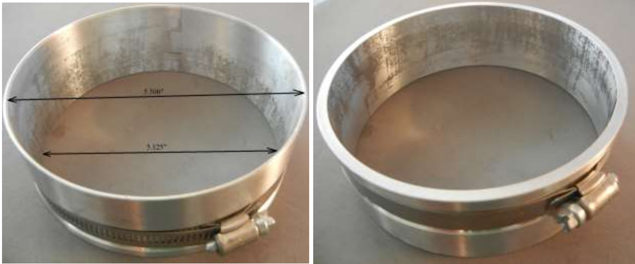
Image 1 & 2 – AX50-92-001 clam-clip compressor tool
