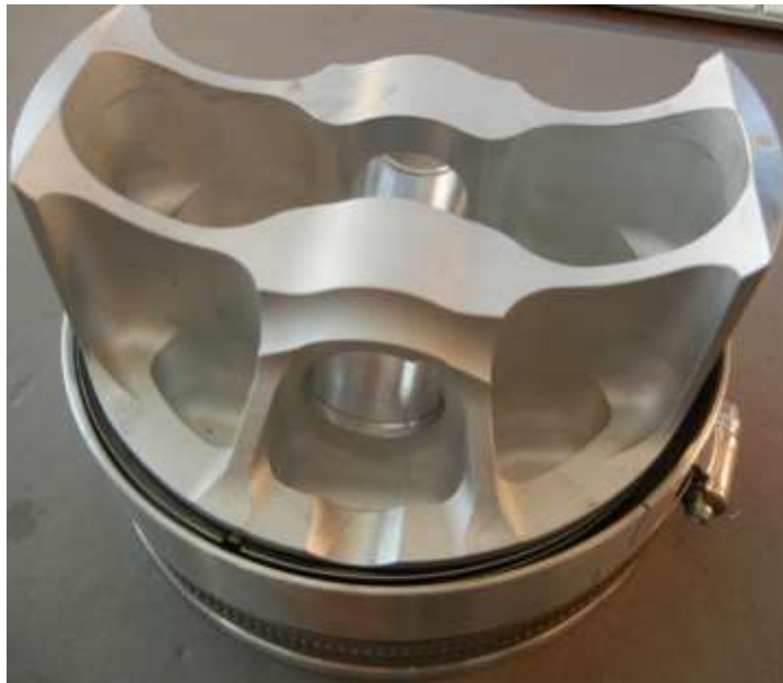
Image 3 – AX40/AX50 piston with rings fitted to AX50-92-001 ring compressor tool
