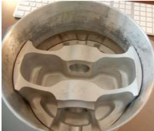
Image 6 & 7 - AX50-92-001 tool in position and piston pushed into cylinder bore.
