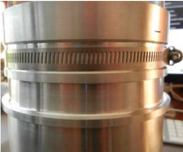
Image 6 & 7 - AX50-92-001 tool in position and piston pushed into cylinder bore.
